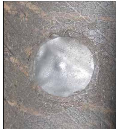
The puncture was "repaired" using only a patch – no plug of any kind was installed – and the damaged area was in no way prepared – the puncture was not reamed out and the innerliner was not cleaned or scraped – to accept the repair, again contrary to advised industry practice. Further, no sealant was used to cover the patch.
